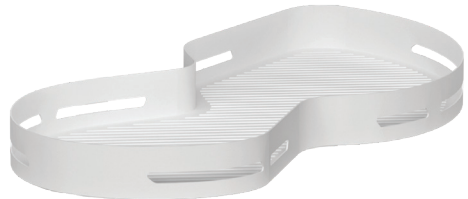
Corner Pull Out Lazy Susan 180 Degrees Right Hand Right Hand Pull Out Shelving Unit with two Trays designed with a swing-out mechanism Suits Blind 900mm wide cabinets Tray Dimensions: 822W x 465D x 60H, Unit Height: 650-750mm 20kg maximum load per tray Colour: White MKLS-180WR
