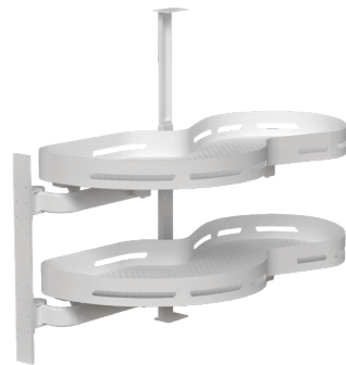
Corner Pull Out Lazy Susan 180 degrees Left Hand Left Hand Pull Out Shelving Unit with two Trays designed with a swing-out mechanism Suits Blind 900mm wide cabinets Tray Dimensions: 822W x 465D x 60H, Unit Height: 650-750mm 20kg maximum load per tray Colour: White MKLS-180WL
